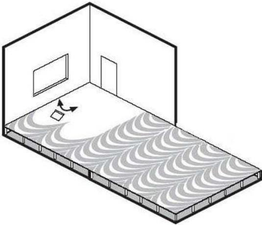
2. Apply the permanent tackifier with a notched trowel in accordance with the instruction of the manufacturer. Allow the adhesive to dry sufficiently.
