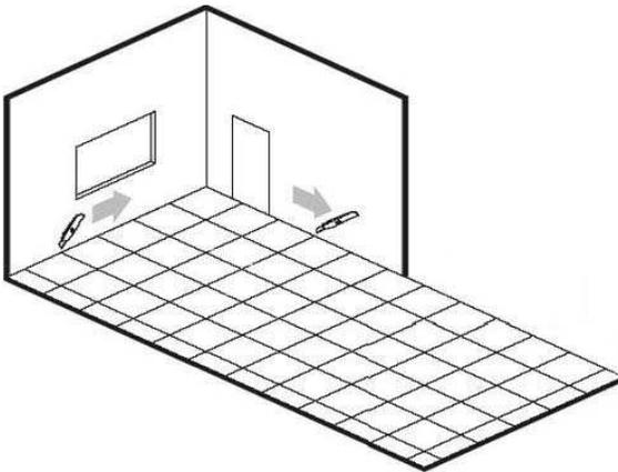
3. Check the uniformity of colour and the absence of defects. The perimeter tiles will require to be trimmed off to be ready for bonding.
