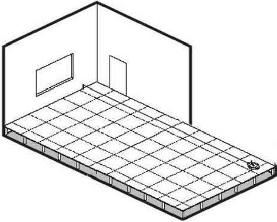
1. Measure the room and mark the centrelines planning the laying in a way to reduce cuts and scraps.
