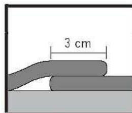
2. Loose lay the rolls (without adhesive) following the marked lines. Rolls must be laid with 3,0 cm overlap along the adjoining edges. Check the uniformity of colour and the absence of defects.
