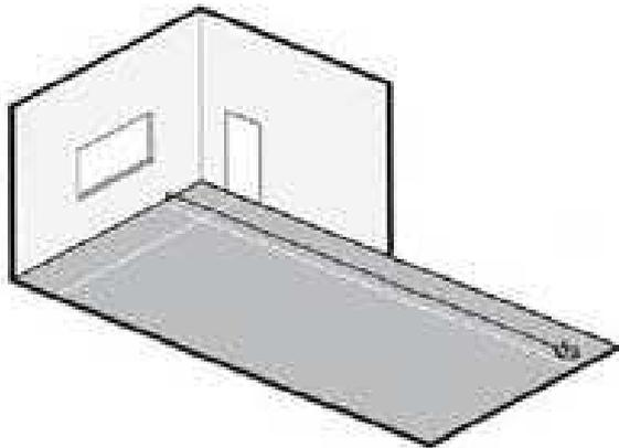
1. Measure the room and mark the centrelines, planning the laying in a way to reduce cuts and scraps.
